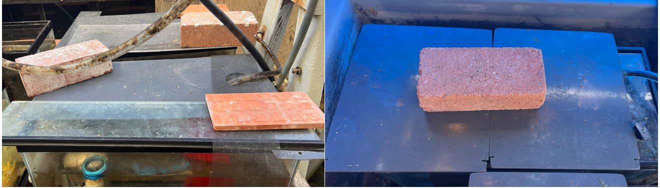
Fig 3. This figure shows 2 different methods of covering tanks to make them “escape-proof”. The first method shows one plastic cover over most of the tank with a 2-inch gap for adding food, which is then covered by a glass panel. Two corners of the tank are held down with bricks and a mesh covering is used where the saltwater hose enters the system. The second method shows one plastic covering with a small hole for the saltwater hose, covered by two smaller plastic coverings held down by a brick. Both methods are suitable but an additional inch of astroturf along the inside of the tank would make it much harder for an octopus to escape.
